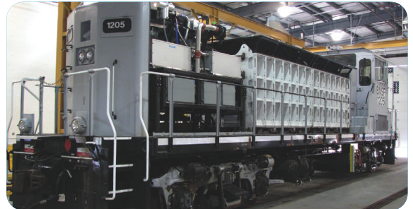
Vehicle Projects created a complex control system for a zero-emission, fuel-cell-powered locomotive.
